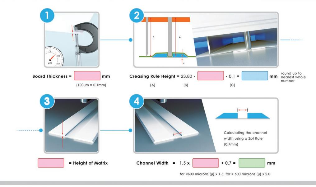
THE WORLD"S MOST ADVANCED CREASING MAKE-READY SYSTEM Fill in the blank spaces above to work out the Matrix Size you require
